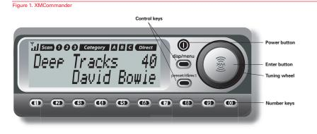
The XMCommander unit has a power button, two control buttons, tuning wheel, enter button and 10 number keys.
